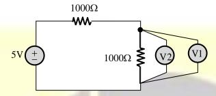
The voltage drop across a resistor is measured using two different voltmeters V1 and V2 at five different time instances and the following values are recorded from V1 and V2.
