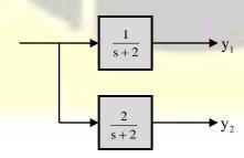
A state space model of the above system in terms of the state vector x and the output vector  $\underline{\mathbf{y}} = [\mathbf{y}_1 \quad \mathbf{y}_2]^{\mathrm{T}} \mathbf{i} \mathbf{s}$
