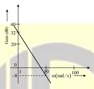
The gain  $(20 \log |G(s)|)$  is 32 dB and -8 dB at 1 rad/s and 10 rad/s respectively. The phase is negative for all  $\omega$ . The G(s) is
