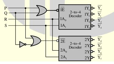
$D_{in}$ ,  $S_0$ ,  $S_1$  and  $S_2$  are to be connected to P, Q, R and S, but not necessarily in this order. The respective input connections to P, Q, R and S terminals should be
