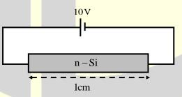
The donor doping concentration  $N_D$  and the mobility of electrons  $\mu_n \operatorname{are10^{16} cm^{-3}} \operatorname{and1000 cm^2 V^{-1} s^{-1}}$ , respectively the average time (in  $\mu$ s) taken by the electrons to move from one end of the bar to other end is \_\_\_\_\_\_.
