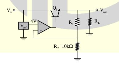
For a load R<sub>L</sub> drawing 200 mA, the maximum power dissipation in Q<sub>1</sub> (in Watts) is \_\_\_\_\_\_.
