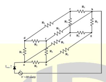
RMS current I<sub>rms</sub> (in mA) through the diode is \_\_\_\_\_.
