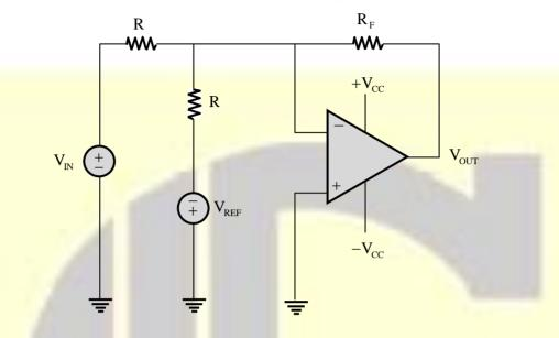
Assuming  $|V_{IN}| \ll |V_{CC}|$  and  $|V_{REF}| \ll |V_{CC}|$ , the condition at which  $V_{OUT}$  equals to zero is
