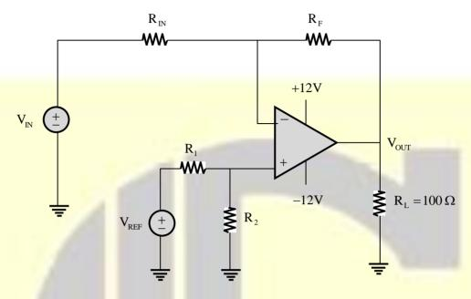
If  $V_{OUT} = 1$  volt for  $V_{IN} = 0.1$  volt and  $V_{OUT} = 6$  volt for  $V_{IN} = 1$  volt, where  $V_{OUT}$  is measured across  $R_L$  connected at the output of this OPAMP, the value of  $R_F/R_{IN}$  is
