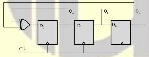
Starting from the initial value of the flip-flop outputs  $Q_2Q_1Q_0 = 111$  with  $D_2 = 1$ , the minimum number of triggering clock edges after which the flip-flop outputs  $Q_2Q_1Q_0$  becomes 100 (in integer) is \_\_\_\_\_.
