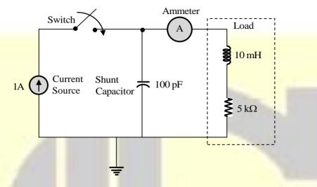
Initially, when the switch is open, the capacitor is discharged and the ammeter reads zero ampere. After the switch is closed, the ammeter reading keeps fluctuating for some till it settles to a final steady value. The maximum ammeter reading that one will observe after the switch is closed (rounded off to two decimal places) is \_\_\_\_\_\_A.
