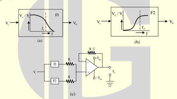
The cut-off frequencies of F1 and F2 are  $f_1$  and  $f_2$  respectively. If  $f_1 < f_2$ , the resultant circuit exhibits the characteristics of a
