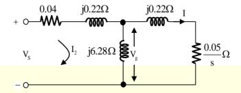
The "air-gap" voltage,  $V_g$  across the magnetizing inductance, is 210V rms, and the slip, is 0.05. The torque (in Nm) produced by the motor is \_\_\_\_\_.
