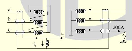
The current transformers (CTs) on low and high voltage sides have a ratio of 500/5. Find the currents  $i_1$  and  $i_2$ , if the fault current is 300A as shown in figure.
