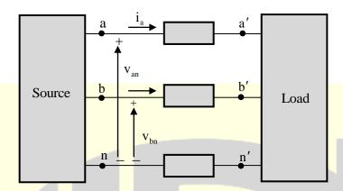
The instantaneous voltage and current ina phase are  $v_{an}=220\sin(100\pi t)V$  and  $i_a=10\sin(100\pi t)A$  respectively. Similarly for phase-b, the instantaneous voltage and current are  $v_{bn}=220\cos(100\pi t)V$  and  $i_b=10\cos(100\pi t)A$ , respectively. The total instantaneous power flowing from the source to the load is
