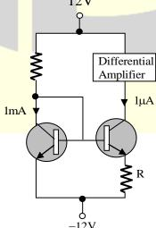
The value of the resistance R in  $k\Omega$  that is required to provide 1  $\mu A$  bias current for the differential amplifier block shown is \_\_\_\_\_.
