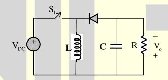
Assume that all components are ideal, inductor current is continuous, and output voltage is ripple free. The range of duty ratio D of the converter for which the magnitude of the steady state output voltage remains constant at 48 V is
