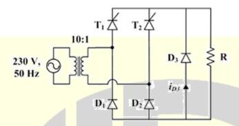
Assume that all devices are ideal. The firing angles of the thyristors  $T_1$  and  $T_2$  are  $90^\circ$  and  $270^\circ$ , respectively. The RMS value of the current through diode  $D_3$  in amperes is \_\_\_\_\_.
