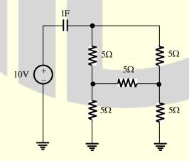
The energy in joules transferred from the DC source until steady state condition is reached equals \_\_\_\_\_\_. (Give the answer up to one decimal place).
