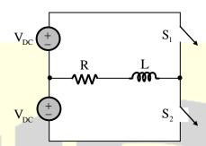
The switch control signal of the converter are generated using sinusoidal pulse width modulation with modulation index, M = 0.6. At 50 Hz, the RL-load draws an active power of 1.44 kW. The value of DC source voltage V<sub>DC</sub> in volts is
