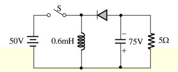
The capacitor is large enough so that the ripple across it is negligible and at steady state acquires a voltage as shown. The peak current in amperes drawn from the 50 V DC source is \_\_\_\_\_\_. (Give the answer up to one decimal place.)
