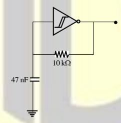
The input capacitance and output resistance of the Schmitt-trigger are negligible. The frequency of the oscillator shown is \_\_\_\_\_Hz.
