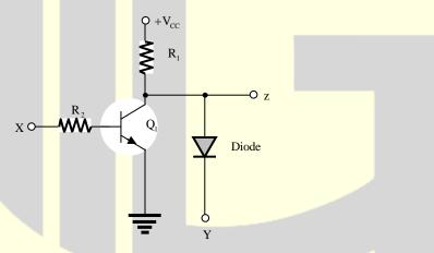
If  $V_{CC}$  is +5V, X and Y are digital signals with 0V as logic 0 and  $V_{CC}$  as logic 1, the Boolean expression for Z is
