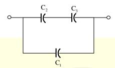
For the interconnection shown below, the maximum safe voltage in volt as that can be applied across the combination, and the corresponding total charge in µC stored in the effective capacitance across the terminals are, respectively.
