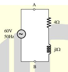
So that the power factor of the parallel combination becomes unity. The value of the capacitance required in  $\mu F$  is \_\_\_\_\_\_.
