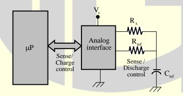
$C_{ref}$  is charged from voltage  $V_L$  to  $V_H$  (by a constant DC voltage source  $V_S$ ), once through  $R_{ref}$  in  $T_{ref}$  seconds and then discharged to  $V_L$ . It is again charged from voltage  $V_L$  to  $V_H$  through  $R_x$  in  $T_x$  seconds.
