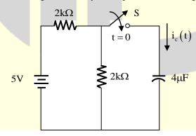
The switch 'S' is closed at t = 0. Two milliseconds after the switch is closed, the current through the capacitor (in mA) is \_\_\_\_\_.
