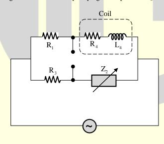
For obtaining balance,  $Z_2$  should consist of element(s)
