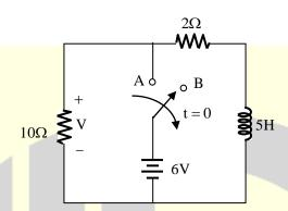
The switch is thrown to position 'B' at time t = 0. The voltage V (volts) across the  $10\Omega$  resistor at time  $t = 0^+$  is \_\_\_\_\_.
