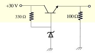
The current (in mA) through the Zener diode is \_\_\_\_\_.
