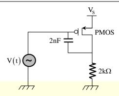
Other parasitic impedances of the MOSFET may be ignored. An external capacitor of capacitance 2 nF is connected across the PMOS transistor as shown. The input impedance in mega ohm as seen by the voltage source is  $\underline{\hspace{1cm}}$  M $\Omega$ .
