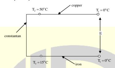
The magnitude of the thermo emf E developed in the circuit shown in the figure, in millivolts is \_\_\_\_\_mV.
