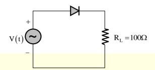
Assuming ideal diode characteristics with zero forward voltage drop and zero reverse current, the average power consumed in watts by the load resistance R<sub>L</sub> is \_\_\_\_\_\_ W.
