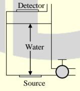
If the height of water in the tank is reduced from 100 mm to 90 mm, the percentage change in the radiation intensity received by the detector, neglecting absorption of the radiation by air, is
