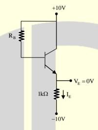
If  $\beta_{dc} = 99$  for the transistor, then the value of  $R_B$  in kilo ohms is \_\_\_\_\_k\Omega .
