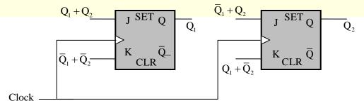
The output sequence of the counter starting from  $Q_1Q_2 = 00$  is
