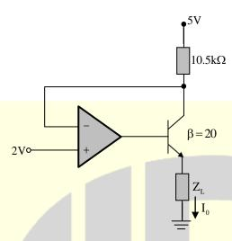
The current  $I_0$  (in  $\mu A$ ) flowing through the load  $Z_L$  is \_\_\_\_\_.
