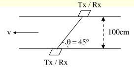
The angle  $\theta$  is 45°. The measured transit times are  $t_1 = 0.9950 \text{ms}$  and  $t_1 = 1.0000 \text{ms}$ . The velocity v (in m/s) in the pipe is (up to one decimal place)\_\_\_\_\_.
