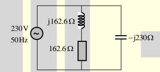
The magnitude of the reactive power (in VAr) supplied by the source is \_\_\_\_\_\_.
