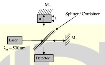
When a dielectric plates of refractive index n = 1.5, of thickness t, is placed in front of the mirror  $M_2$ , a dark fringe is observed on the detector. When the dielectric plate is removed without changing the position of the mirrors  $M_1 \& M_2$ , a bright fringe is observed on the detector. The minimum thickness t(in nm) of the dielectric is \_\_\_\_\_\_.
