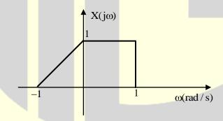
Let  $y(t) = x(t) + e^{jt} x(t)$ . The value of Fourier transform of y(t) evaluated at the angular frequency  $\omega = 0.5$  rad/s is
