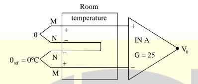
If the output  $V_0$  is 96 mV, then the value of  $\theta$  (in °C) is\_\_\_\_\_
