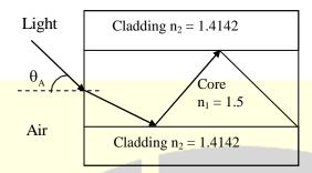
The maximum value of  $\theta_A$  (in degrees) for which the incident light from air will be guided in the optical fiber is  $\pm$  \_\_\_\_\_.
