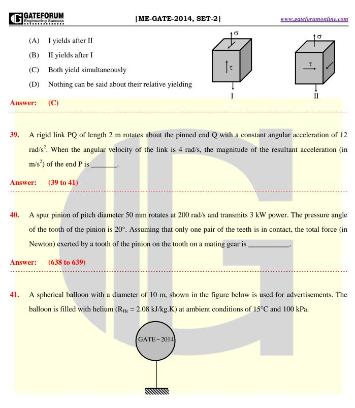
Assuming no disturbances due to wind, the maximum allowable weight (in newton) of balloon material and rope required to avoid the fall of the balloon ( $R_{air} = 0.289 \text{ kJ/kg.K}$ ) is \_\_\_\_\_.
