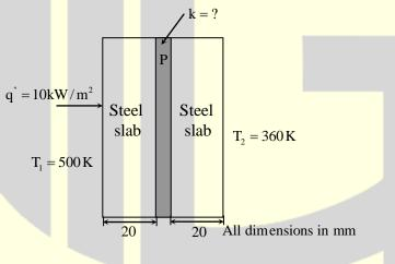
The boundary temperatures of the slabs are indicated in the figure. Assume thermal conductivity of this steel is 10 W/m.K. considering one-dimensional steady state heat conduction for the configuration, the thermal conductivity (k, in W/m.K) of material P is \_\_\_\_\_\_.
