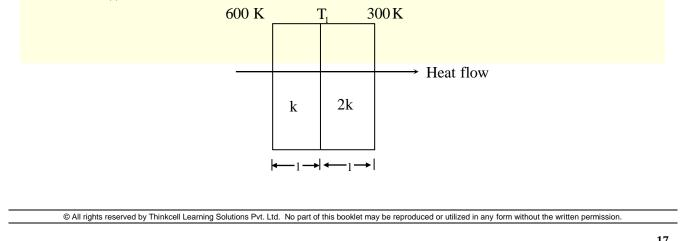
The conductivity of one section is k and that of the other is 2k. The left face of the wall is at 600 K and the right face is at 300 K. The interface temperature Ti (in K) of the composite wall is \_\_\_\_\_.
