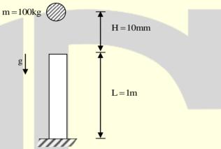
If  $g = 10 \text{m/s}^2$ , the maximum compression of the elastic bar is \_\_\_\_\_ mm.
