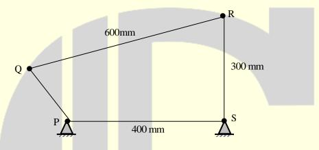
For the mechanism to be crank-rocker mechanism, the length of the link PQ can be
