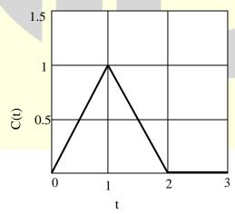
The mean residence time in the reactor, rounded to 1 decimal place, is \_\_\_\_\_\_s.
