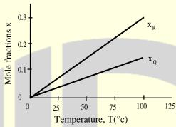
The mole fractions of product components  $(x_Q \text{ and } x_R)$  were found to vary linearly with temperature as given in the figure.
