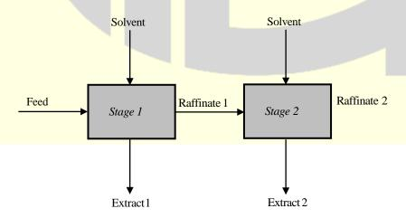
Components B and C are immiscible, 60% of A in the feed is extracted in Stage 1. The equilibrium relation is given by  $Y^*=1.5X$  where
