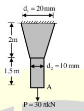
Both bars are made of same material with the modulus of elasticity,  $E = 2 \times 10^5$  MPa. When subjected to a load  $P = 30\pi$  kN, the deflection at point A is \_\_\_\_\_ mm.
