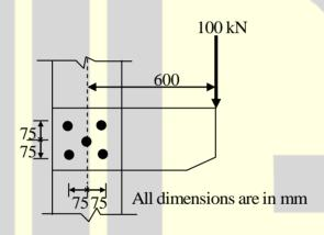
The maximum force for which the bolts should be designed is \_\_\_\_\_ kN.
