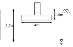
Using Terzaghi's bearing capacity equation and a factor of safety  $F_s$ = 2.5, the net safe bearing capacity (expressed in kN/m<sup>2</sup>) for local shear failure of the soil is \_\_\_\_\_\_.
