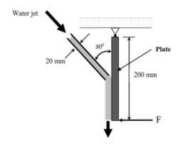
Consider g as 9.81 m/s<sup>2</sup> and neglect the self-weight of the plate. The force F (expressed in N) required to keep the plate in its vertical position is \_\_\_\_\_\_\_.
