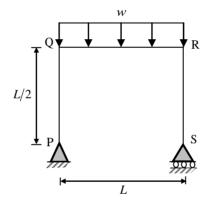
The bending moment in the beam at the joint 'Q' is
