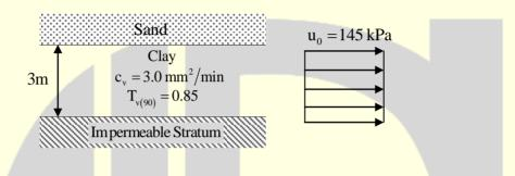
For the given ground conditions, the time (in days, rounded to the nearest integer) required for 90% consolidation would be \_\_\_\_\_
