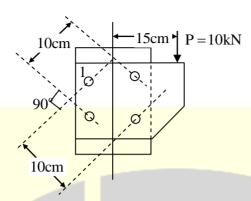
The resultant force (in kN, up to one decimal place) in the bolt 1 is\_\_\_\_\_
