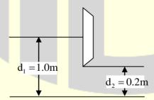
It is observed that the depth of flow is 1.0 m upstream of the gate, while the depth is 0.2 m downstream of the gate. Assuming a smooth flow transition across the sluice gate, i.e., without any energy loss, and the acceleration due to gravity as 10 m/s<sup>2</sup>, the discharge (in m<sup>3</sup>/s, up to two decimal places) passing under the sluice gate is\_\_\_\_\_.
