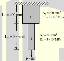
Segments 1 and 2 have cross-sectional area of  $100 \text{ mm}^2$  and  $60 \text{ mm}^2$ , Young's modulus of  $2 \times 10^5 \text{ MPa}$  and  $3 \times 10^5 \text{ MPa}$ , and length of 400 mm and 900 mm, respectively. The strain energy (in N-mm, up to one decimal place) in the bar due to the axial load is \_\_\_\_\_\_.
