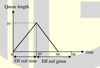
At time t = 0, the light has just turned red. The effective green time is 36 seconds, during which vehicles discharge at the saturation flow rate, s (in vph). Vehicles arrive at a uniform rate, v (in vph), throughout the cycle. Which one of the following statements is TRUE?
