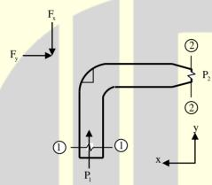
A pressure of 140 kPa is measured at section 1-1. The inlet diameter marked at section 1-1 is  $\frac{27}{\sqrt{\pi}}$  cm, while the nozzle diameter marked at section 2-2 is  $\frac{14}{\sqrt{\pi}}$  cm. Assume the following:
