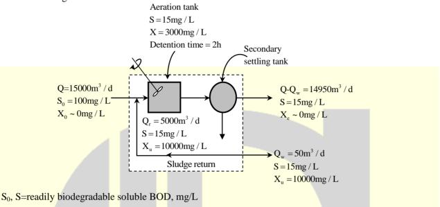
Q, Q<sub>r</sub>, Q<sub>w</sub>=flow rates,  $m^3/d$
