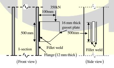
The maximum resultant stress (in MPa, round off to 1 decimal place) on the fillet weld along the vertical plane would be \_\_\_\_\_.
