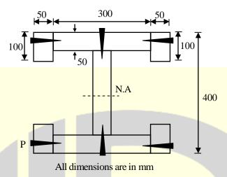
The beam is symmetrical about the neutral axis (N.A.) shown, and the moment of inertia about N.A. is  $1.5 \times 10^9 \text{mm}^4$ . Considering that the nails at the location P are spaced longitudinally (along the length of the beam) at 60 mm, each of the nails at P will be subjected to the shear force of
