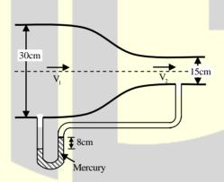
When the water flow, the differential manometer shows a deflection of 8cm of mercury (Hg). The value of specific gravity of mercury and water are 13.6 and 1.0, respectively. Consider the acceleration due to gravity.  $g = 9.81 \text{ m/s}^2$ . Assuming frictionless flow, the flow rate (in  $m^3/s$ , rounded off to 3 decimal places) through the duct is \_\_\_\_\_.
