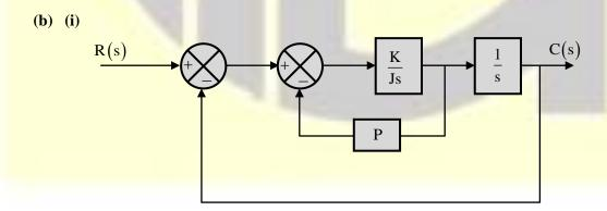
Determine the value of K and P of the closed loop system shown in the figure, so that the maximum overshoot in unit step response is 25% and the peak time is 2 sec. Assume that  $J = 1 \text{ kg-m}^2$
