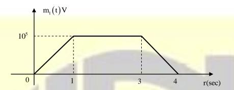
Consider a message signal  $m_1(t)$  as shown and message signal  $m_2(t) = \sin c(2 \times 10^4 t)$ , in volts.
