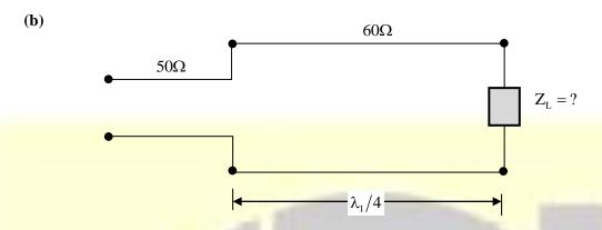
Find the load impedance which can be matched to a  $50\Omega$  transmission line with a quarter wave line (at  $f = f_1$ ) of characteristics impedance  $60\Omega$ . If the frequency is doubled (at  $f = 2f_1$ ), what will be the VSWR on  $50\Omega$  line?
