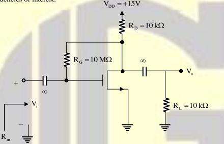
The effect of channel length modulation on the dc operating point can be neglected.
