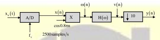
In this system,  $H(\omega)$  is a low-pass filter with a discrete cut-off frequency equivalent to  $f_c$  = 125 Hz (normalized w.r.t. the sample rate at the point in the block diagram). Determine and sketch the spectra of  $X(\omega_x), W(\omega_w), V(\omega_v)$  and  $Y(\omega_y)$  w.r.t.  $\omega_x, \omega_w, \omega_v$  and  $\omega_y$  respectively for  $-\pi < \omega < \pi$ .
