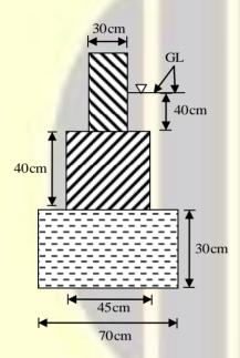
The wall and first footing are of randomrubble masonry in cement mortar; and the lowest part of the foundation is of mass rubble in cement mortar. The total volume of the 40 cm deep footing for the whole building is, nearly
