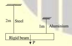
two rods of steel and aluminium, 2 m and 1 m long, having values of cross sectional areas 100 mm2 and 200 mm2, and young's modulus of 200 GPa and 100 GPa, respectively. A load P is applied as shown in the figure above: If the rigid beam is to remain horizontal then
