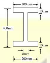
If the permissible stress is 150N/mm<sup>2</sup>, the bending moment M will be nearly
