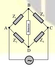
$Z_1 = 100 \Omega$  with phase angle of  $60^{\circ}$ ,  $Z_2 = 300 \Omega$ with phase angle of  $0^{\circ}$ , and  $Z_3 = 50 \Omega$  with
