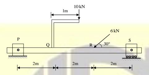
The bending moment, in Nm, at point R is \_\_\_\_\_\_.
