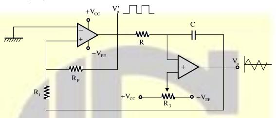
(ii) Design a square wave generator as shown in the figure below, so that duty cycle is 50% and  $f_o = 2.5$  kHz. Assume  $V_{CC} = 12V$  and  $C = 0.1 \mu F$ .
