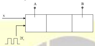
The frequency of signal x is  $f_s$  and the shift register is clocked at the positive edge of  $2f_s$ . The time offset between A and B is
