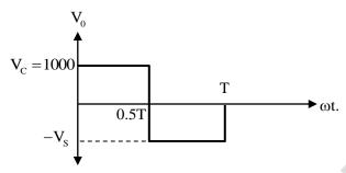
Since current is having fundamental component only. Therefore to calculate active power, we have to consider  $V_0$  fundamental component only
