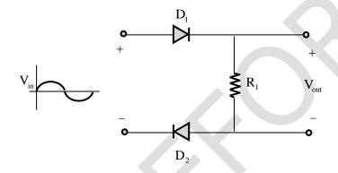
For +ve half cycle, both the diodes will be "ON' and these are ideal diodes, so it will act as short circuit.
