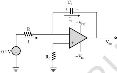
$$\begin{split} I_1 &= I_2 \\ \frac{0.1 - 0}{R_1} &= -C_1 \frac{dV_o}{dt} \\ \frac{dV_o}{dt} &= \frac{-0.1}{R_1 C_1} \\ V_o &= \frac{-0.1}{R_1 C_1} \int dt = -0.1 \left(\frac{t}{R_1 C_1}\right) \end{split}$$
