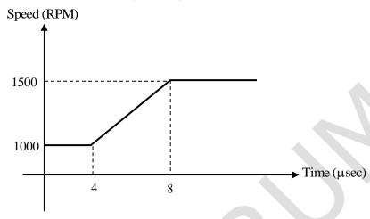
& we need to calculate the energy, in Joules consumed by the motor during the speed change.
