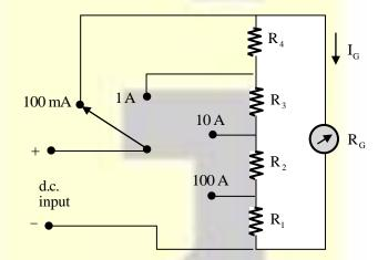
What are the values of resistances  $R_1$ ,  $R_2$ ,  $R_3$  and  $R_4$ , if the shunt resistances are connected as shown in the figure?
