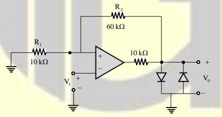
**2.** In the above circuit, if  $\mathbf{R}_1$  is open circuit and  $\mathbf{R}_2$  is short-circuit, redraw the characteristics.
