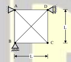
Structure II: Pin-jointed truss, with hinge support at A, and rollers at B and D.
