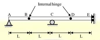
Structure I: Beam with hinge support at A, roller at C, guided roller at E, and internal hinges at B and D.
