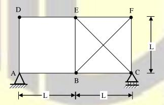
Structure III: Pin-jointed truss, with hinge support at A and roller at C.
