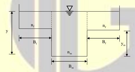
B<sub>m</sub> – Bottom width of main channel
