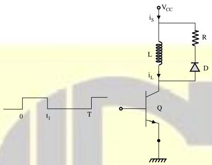
For the figure shown above, the transistor 'Q' is excited by a pulse of duration ' $t_1$ ' with a periodicity of  $\frac{1}{T}$
