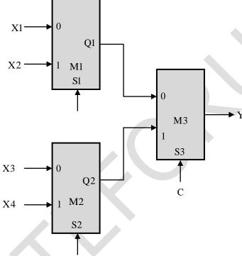
For an instance of inputs X1 = 1, X2 = 1, X3 = 0 and X4 = 0, the number of combinations of A, B, C that given the output Y = 1 is \_\_\_\_\_.
