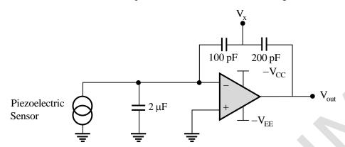
When the piezoelectric sensor generates a charge  $q_p$ , the resulting change in voltage  $V_x$  is -2V. Then the corresponding change in the voltage  $V_{out}$  is \_\_\_\_\_\_ V (rounded off to nearest integer).
