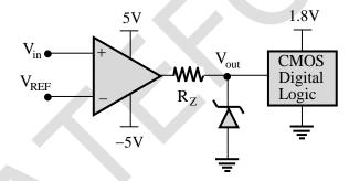
The CMOS digital logic circuit has input impedance. Assume that opamp is ideal. A 1.8 V Zener diode with a minimum Zener current of 2 mA is used. The corresponding maximum value of resistance  $R_Z$  is  $k\Omega$ . (rounded off to one decimal place).
