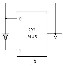
If S is set to 1 then the output Y is \_\_\_\_\_
