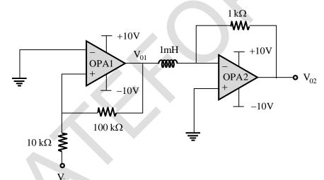
Assume that the initial inductor current is 0A. The input voltage (V<sub>i</sub>) is a triangular signal with peak voltages of  $\pm 2$  V and time period of 8  $\mu$ s. Which one of the following statements is true?
