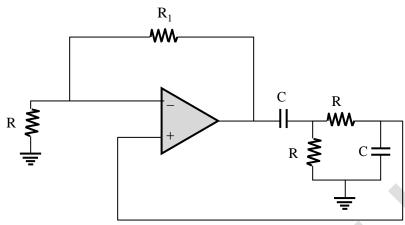
If the circuit is to show sustained oscillations, the respective values of  $R_1$  and the corresponding frequency of oscillation are \_\_\_\_\_\_.
