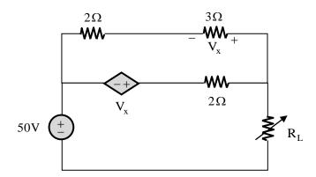
We know value of  $R_L$  for maximum power transfer is  $R_{th}$
